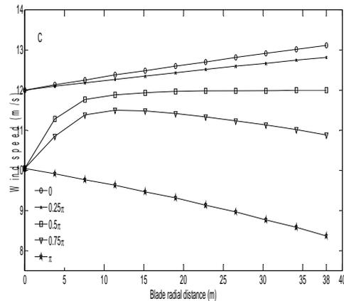
Figure 2. Wind speed for different  $h$  ( $v_h = 12$  m/s,  $\alpha = 0.2$ ,  $R = 38$  m,  $a = 1.5$  m,  $x = 2.9$  m): (A)  $h = 50$  m. (B)  $h = 60$  m. (C)  $h = 70$  m.
