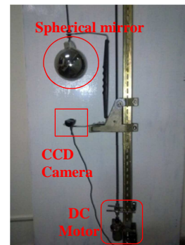
Figure 2. The catadioptric omnidirectional vision system.
