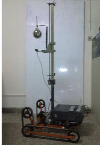
Figure 3. View of the ESCALADE360 Robot and the embedded omnidirectional camera system.
