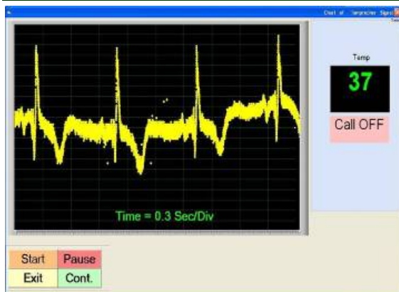
Figure(6) GUI screen showing ECG signal, temperature, and Nurse call OFF for patient
