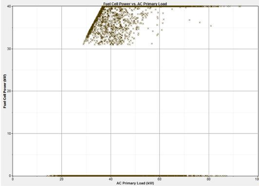
Fig 3 gives the variation of fuel cell power in KW versus the AC primary load in KW Fig 4.
