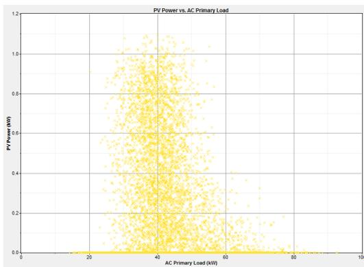
Fig 4. Photo Voltaic power in KW versus the AC primary load in KW
