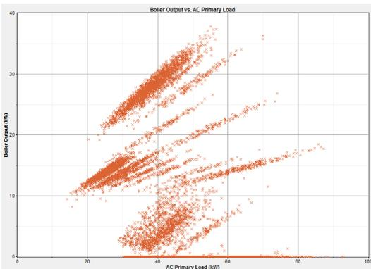
Fig 5. Boiler output (KW) versus the AC primary load in KW
