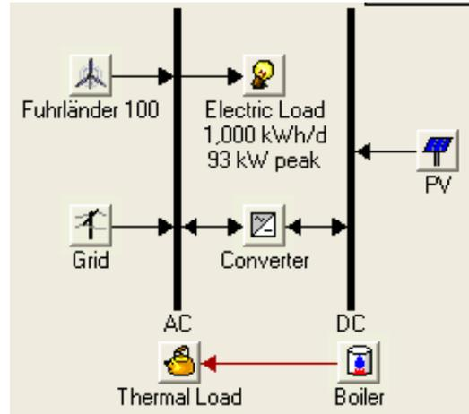
Fig.6. Block diagram of the hybrid (Wind-PV) with AC Grid (without fuel cell)
