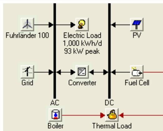
Fig. 1. Block diagram of the proposed hybrid Wind-PV-Fuel cell DG with AC Grid
