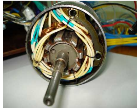
Figure 1. SRM. with 12/8 configuration
