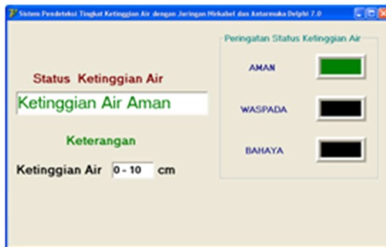
Figure 10. Information is being displayed on PC when the water level at 0 - 10 cm
