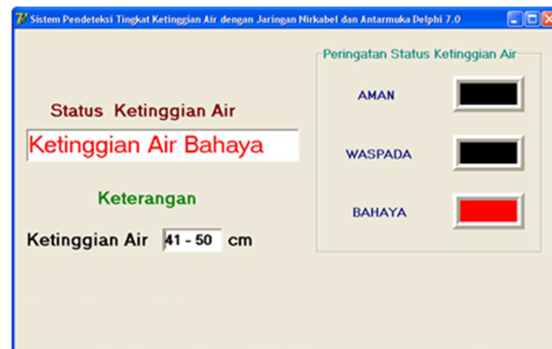
Figure 12. Information is being displayed on PC when the water level at 41 - 50 cm
