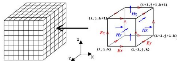
Figure 2 Discretization of the computational domain into Yee cell's for field computation
