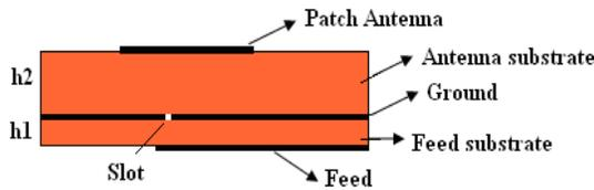
Figure 1 Geometry of Aperture coupled antenna
