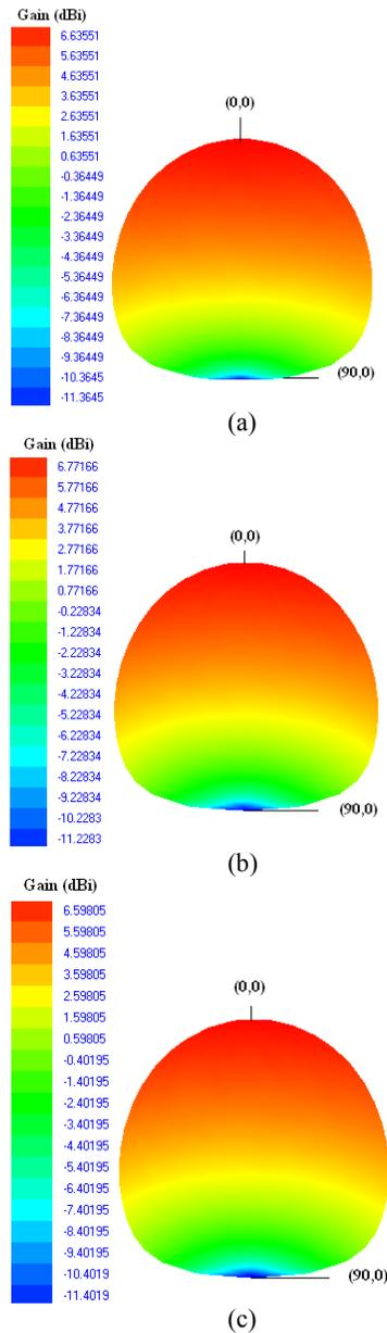
Figure. 4 3D radiation pattern of the proposed antenna at (a) 60 GHz, (b) 61 GHz and (c) 63 GHz
