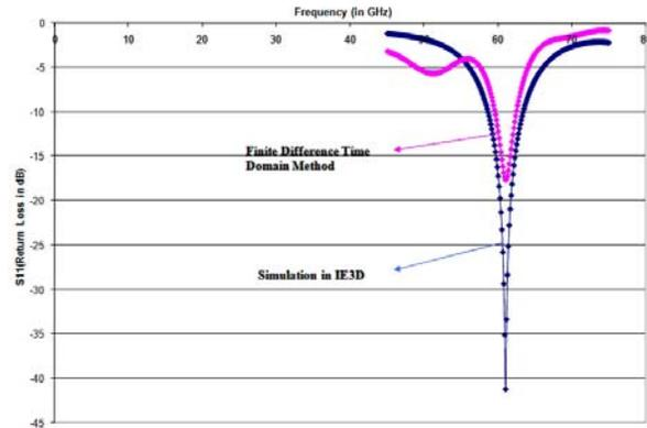
Figure. 6 Comparison of FDTD and simulation results of the proposed antenna.
