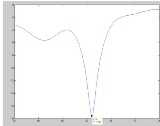
Figure. 3 Return loss characteristics of the proposed antenna by FDTD method
