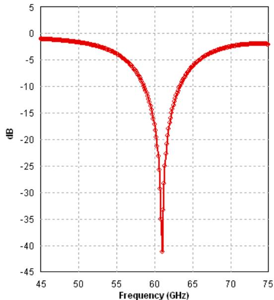
Figure. 4 Return loss characteristics of the proposed antenna
