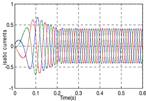
Figure12: Performance of the PMSM with speed ramping up and down.
