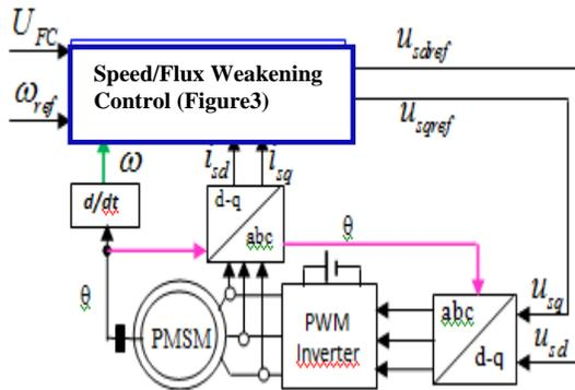
Figure4: Block diagram of speed-regulated PMSM drive system with SFWC in the flux-weakening region
