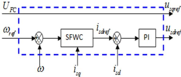
Figure3. Block diagram of flux-weakening control with SFWC
