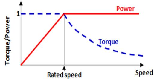
Figure1: Typical characteristics curve of torque/power vs speed of PMSM
