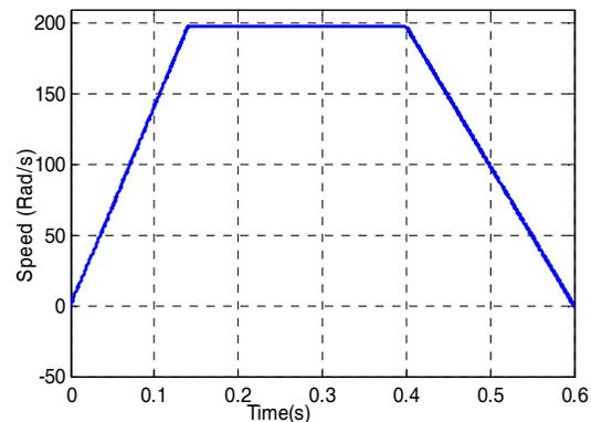
Figure5: Performance of the PMSM with speed ramping up and down.
