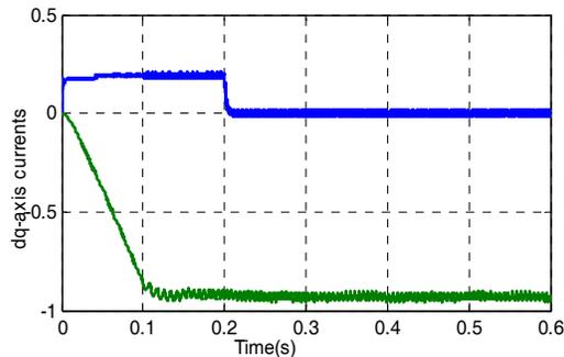
Figure13: Performance of the PMSM with speed ramping up and down.
