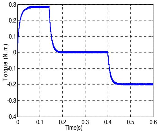
Figure8: Performance of the PMSM with speed ramping up and down.
