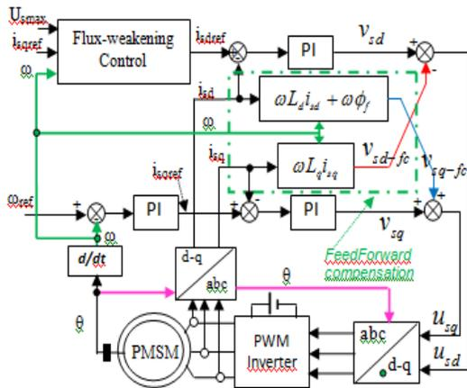
Figure 2. Bloc diagram of speed regulated PMSM drive system with flux weakening control
