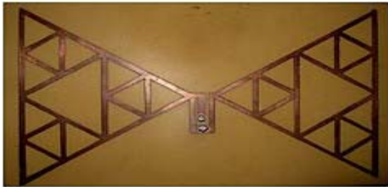
Fig. 1 Representation of a micro-tape fractal antenna.
