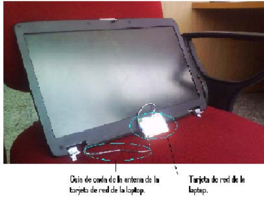
Fig. 7 Photo of the net card and the wave guide of a laptop
