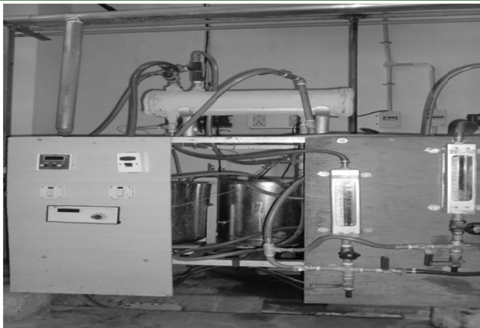
Figure 2: 1-2 Shell and Tube Heat Exchanger with accessories.
