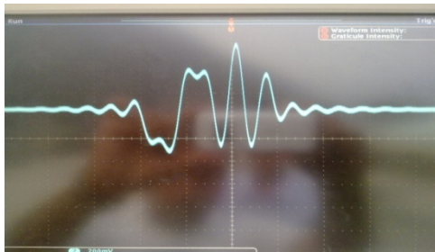
Fig. 3: Generated 11-Bit Barker Code Pattern at the output of the AWG
