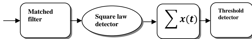
Fig. 1 Simplified block diagram of a square law detector and non-coherent integration
