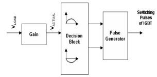
Figure 4: Block diagram of control method for HVC
