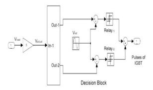
Figure 5: Simulink Model of HVC
