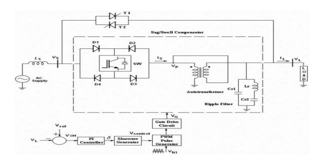
Figure 2: Block Diagram of Voltage Sag Mitigation using IGBT Switching - PWM control
