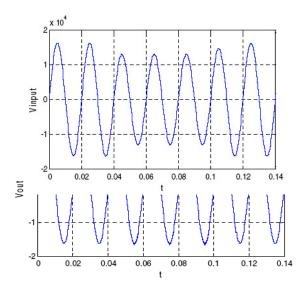
Figure 6: Input voltage having 20% sag given to both schemes
