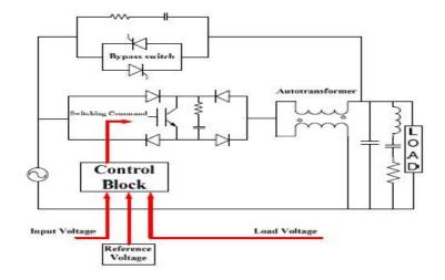
Figure 3: Block Diagram of Voltage Sag Mitigation using IGBT Switching -for HVC control
