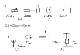
Figure 1 Block diagram of the considered FACTS devices: a) TCSC b) TCPST c) UPFC d) SVC
