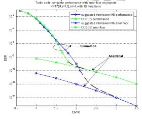
Figure 7. perfornmance comparison for CCSDS turbo code with suggested interleaver M6,K=1784, r=1/2 (better in error floor region)
