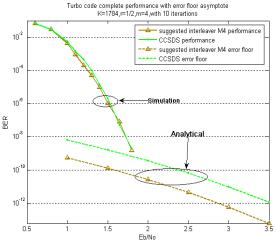
Figure 8. performance comparison for CCSDS turbo code with suggested interleaver M4,K=1784, r=1/2 (better in water fall region)
