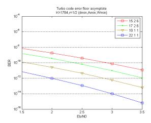
Figure 6. Analytical error floor Asymptote for K=1784, r=1/2 for different parameter (d<sub>min</sub>,A<sub>min</sub>,W<sub>min</sub>).
