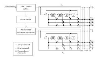
Figure 1 CCSDS turbo code encoder.
