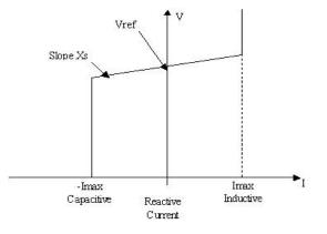
Figure 2. V-I characteristics of STATCOM
