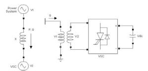
Figure 1. Schematic representation of STATCOM
