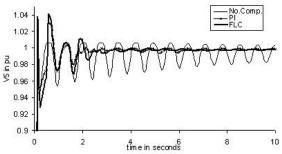
Figure 11: Voltage at Bus – 5 for 3-Ph Short-circuit at Bus – 7
