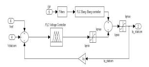
Figure 4: STATCOM model with Combined FLC Voltage Regulator and FLC Bang-Bang controller block diagram
