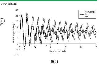
Figure 8. Rotor angle Oscillations of (a) Generator-2, and (b) Generator-3 with respect to Generator-1 for 3-Ph Short circuit at Bus – 7
