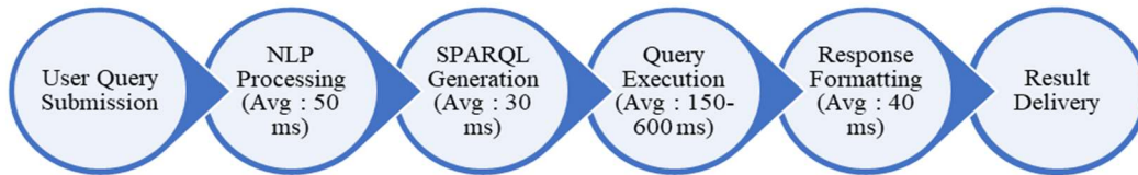
Figure 4 Query Processing Pipeline with Time Distribution
