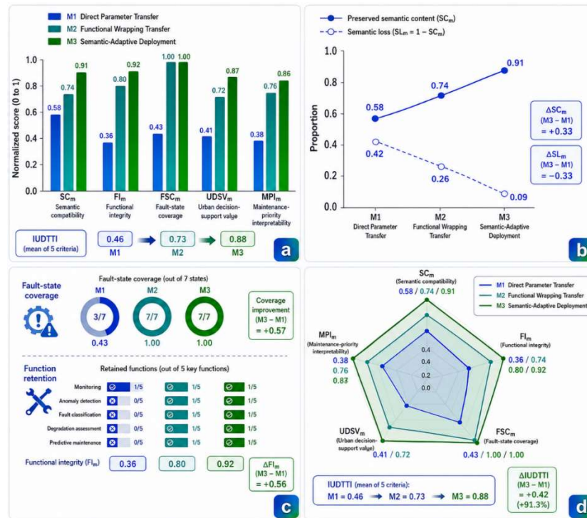
a – Comparison of formalized transfer metrics for M1, M2, and M3; b – Dynamics of semantic compatibility and semantic loss between mechanisms M1, M2, and M3; c – Fault-state coverage and preservation of Industrial Pump Twin functions after semantic-adaptive deployment; d – Profile of IUDTTI and key transfer quality criteria for M1, M2, and M3
