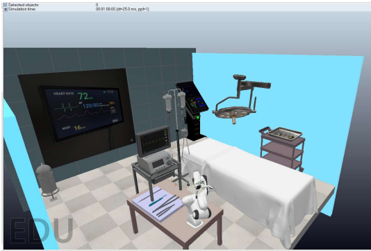
Figure 2: High-Fidelity Surgical Workspace in Coppelia sim Showing Robotic Arm, Vital Monitors, Lighting System, And Patient Bed.
