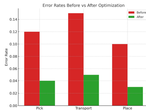
Figure 7: Error-rate comparison for pick, transport, and placement phases before and after optimization.
