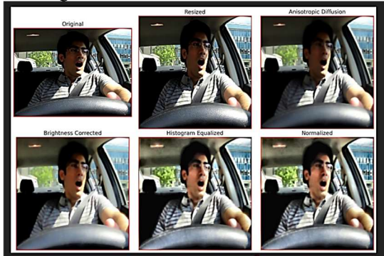
Fig. 2. Sequential pre-processing pipeline applied to driver facial images
