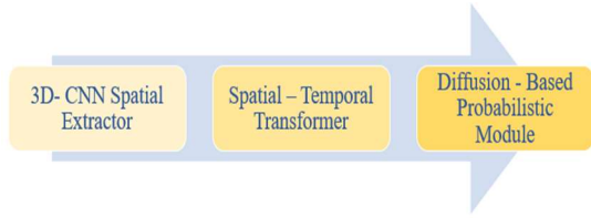
Fig. 4: Three-part architecture consisting of 3D-CNN, transformer and diffusion module
