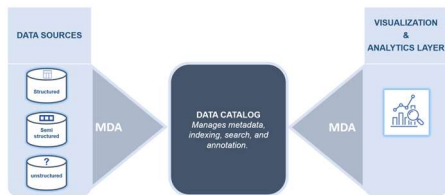
Figure 11: Automated Data Catalog architecture
