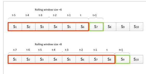
Figure 6: A sample of time series data sliding window (rolling window size of 6 and 8).
