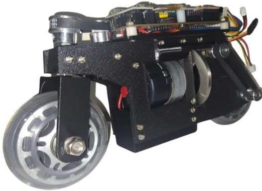
Figure 11. Final design of the autonomous motorcycle prototype
