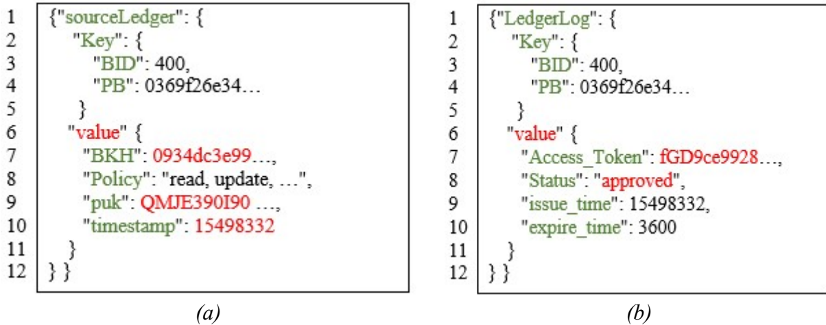
Figure 6. The content of different block headers in the blockchain. (a) Content of the requested block header from ledger source to add new block into blockchain platform based on a JSON format. (b) Content of the response block header from ledger log to source ledger based on a JSON format.
