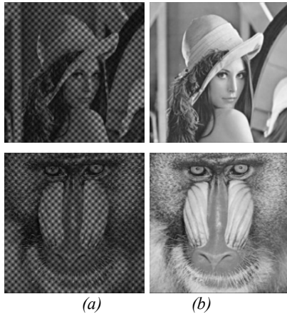
Figure 7: Visual comparison of images, (a) Hexagonal grid image, (b) Gabor filtered Hexagonal Grid image
