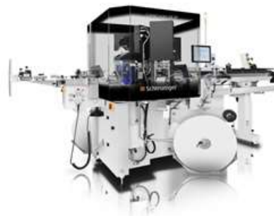
Figure 2: Cutting machine Crimp Center 64 SP
