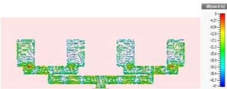
Figure 8(E): Current Distribution At A Frequency Of 54 Ghz.
