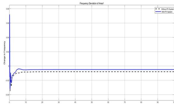
Figure 3: Frequency Deviation in Area 1 of Two Area Interconnected Microgrid system
