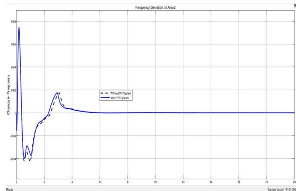
Figure 10: Frequency Deviation in Area 1 and Area 2 of Two Area Interconnected Microgrid system using PI controller
