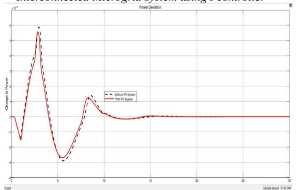
Figure 14: Tie-line power deviation in Interconnected Microgrid system with I Controller
