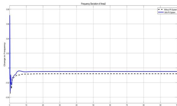
Figure 4: Frequency Deviation in Area 2 of Two Area Interconnected Microgrid system
