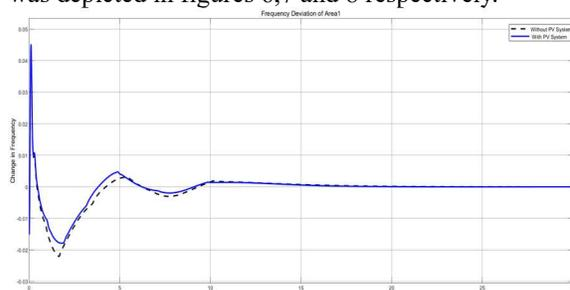
Figure 6: Frequency Deviation in Area 1 and Area 2 of Two Area Interconnected Microgrid system using PID controller
