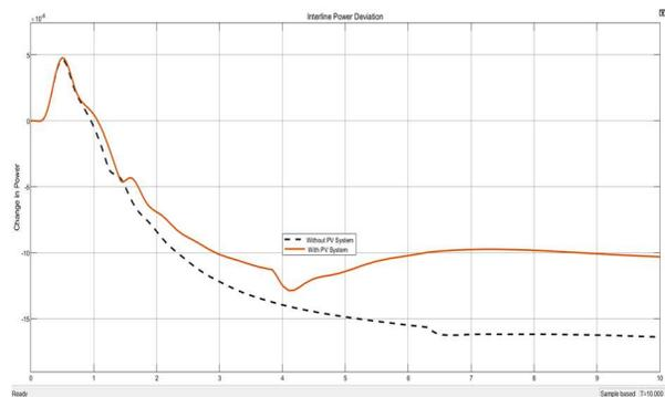
Figure 5: Tie-line power change in Interconnected Microgrid system
