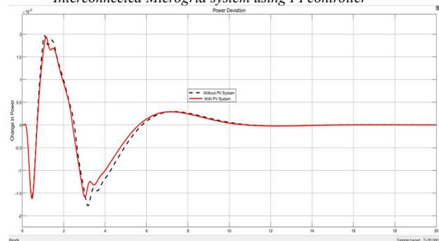
Figure 11: Tie-line power deviation in Interconnected Microgrid system with PI Controller
