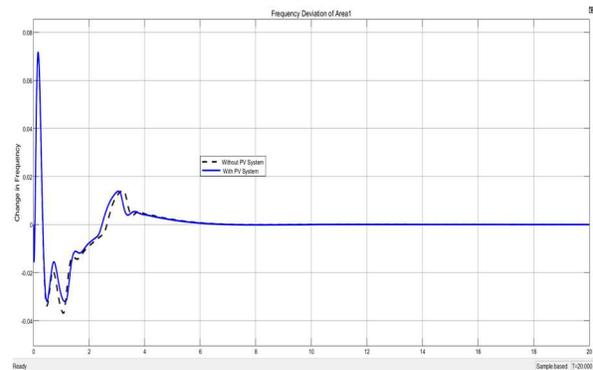
Figure 9: Frequency Deviation in Area 1 and Area 2 of Two Area Interconnected Microgrid system using PI controller
