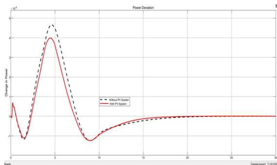
Figure 8: Tie-line power deviation in Interconnected Microgrid system with PID Controller
