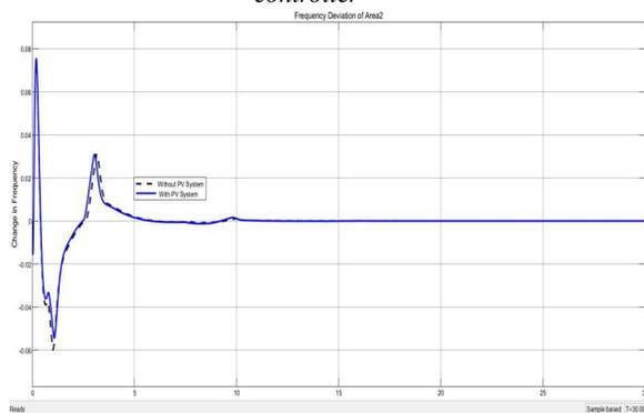
Figure 13: Frequency Deviation in Area 2 of Two Area Interconnected Microgrid system using I controller
