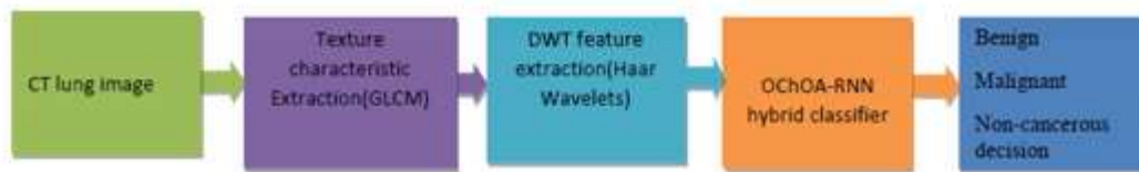
Figure.1 Block diagram of OChOA-RNN: Oppositional based Chimp Optimization Algorithm (OChOA) in association with Recurrent Neural Network (RNN) Hybrid
