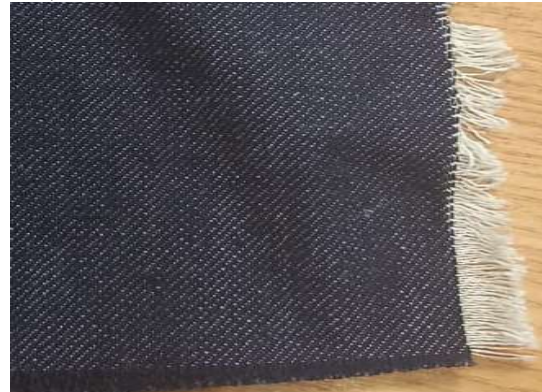
Figure 1. 100% cotton Jean fabric Weave: 4-ply twill, straight cord effect
