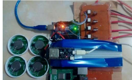
Figure 13: BLE iBeacon and BME280 5V Temperature and Humidity Sensor Calibration
