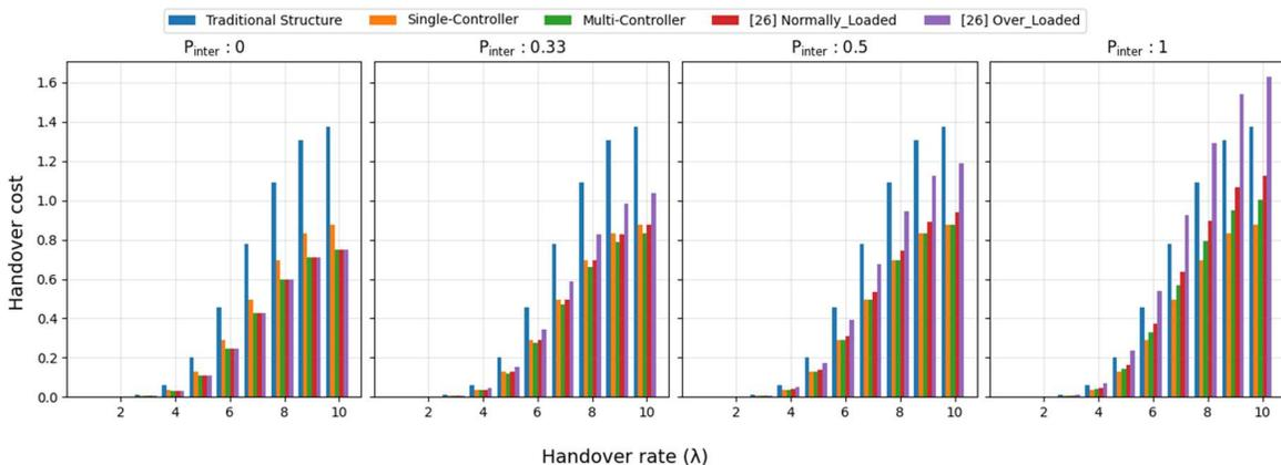
Figure 7: Handover Cost Comparison Of Various Network Structures With Different  $P_{Inter}$  Values ( $K=10$ ).
