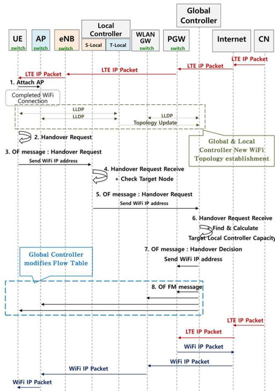
Figure 5 : The Procedure Of Handover From LTE To Wifi With A Global Controller In Multi-Controller Structure.
