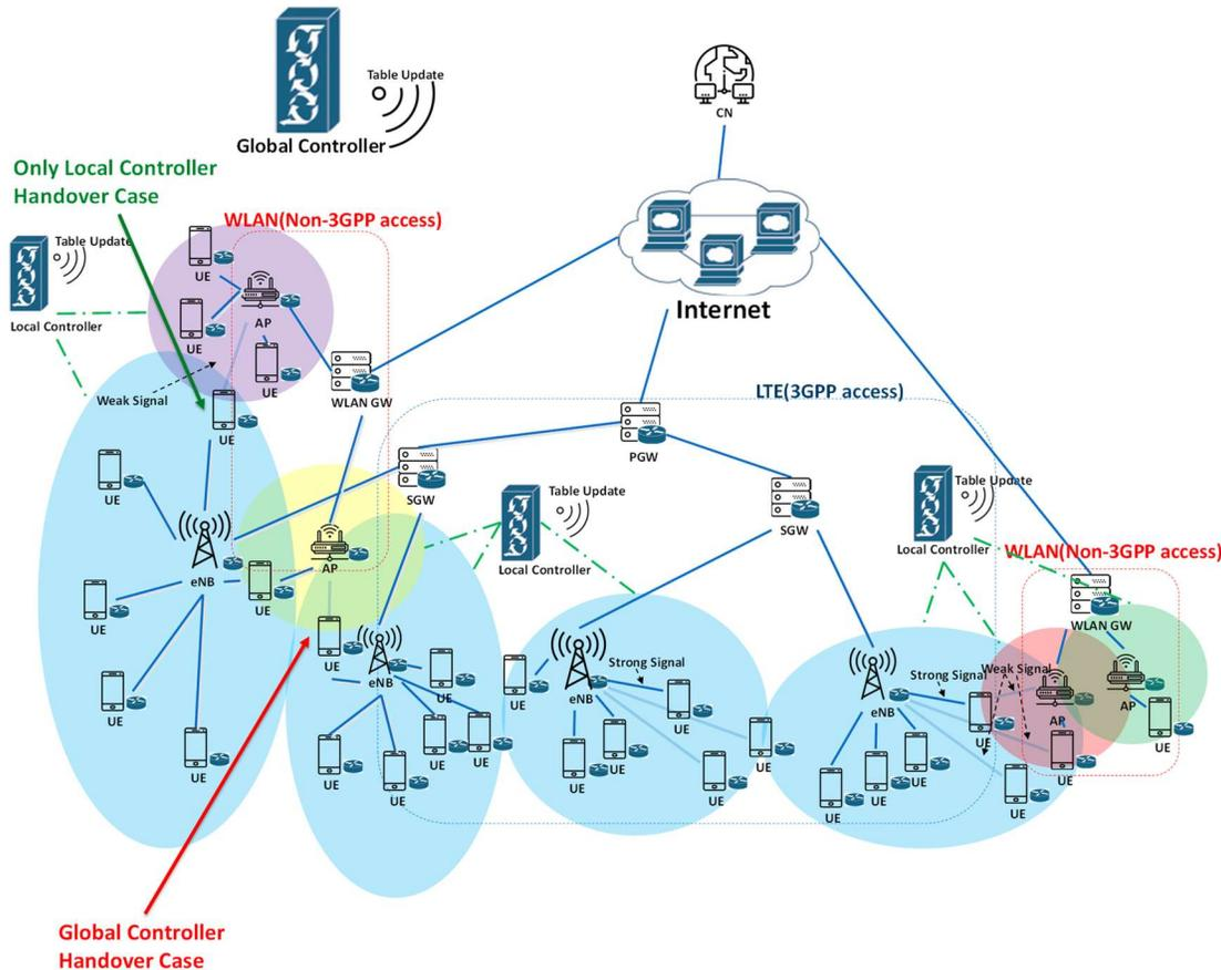
Figure 1: LTE and WiFi interworking architecture with loosely-coupled connections with multi-controllers.
