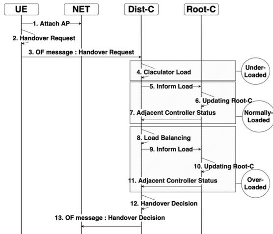
Figure 6 : A Handover Procedure Based On [26].
