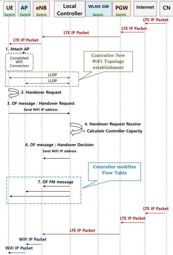
Figure 4 : The Procedure Of Handover From LTE To Wifi Without A Global Controller In Multi-Controller Structure.
