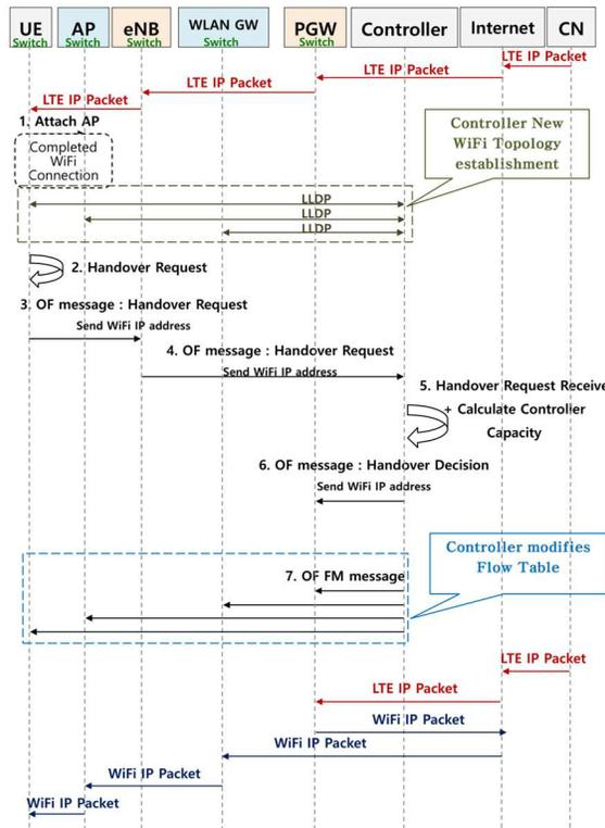
Figure 3 : The Procedure Of Handover From LTE To Wifi In Single-Controller Structure.
