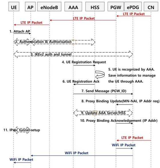
Figure 2 : The Procedure Of Handover From LTE To Wifi In Traditional Structure.
