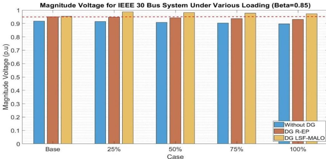
Figure 5: Minimum voltage magnitude under several loadings (beta = 0.85)
