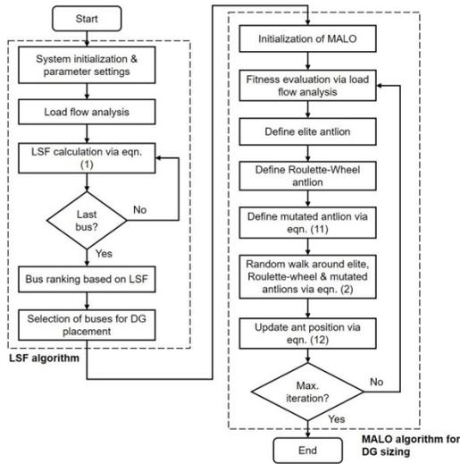
Figure 1: Flowchart for the proposed LSF-MALO algorithm
