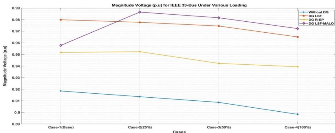
Figure 4: Minimum voltage magnitude under several reactive loadings (base case to 100% loading)
