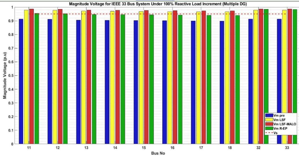
Figure 3: Voltage profile for ten buses with the lowest voltage magnitude (100% loading)
