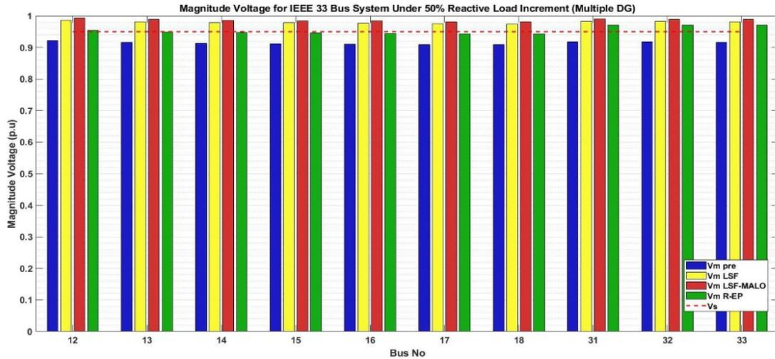
Figure 2: Voltage profile for ten buses with the lowest voltage magnitude (50% loading)
