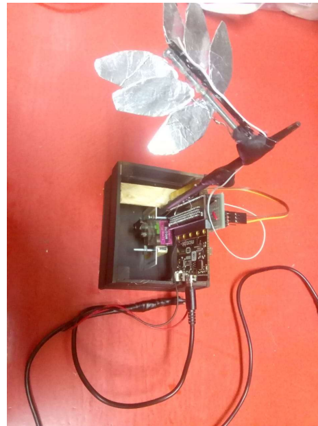
Figure 26: Implementation of connection of sensors to Microbit.
