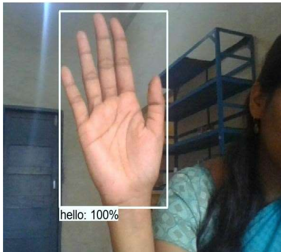
Figure 13: Hello sign detected in real-time using SSD MobileNet V2
