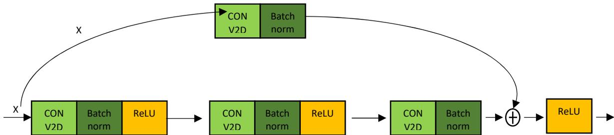
Figure-4. Skipping The Convolutional Layers
