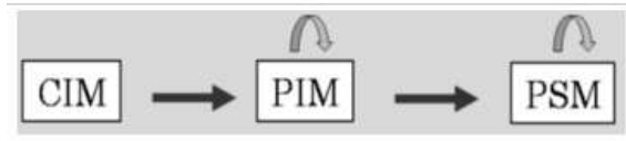
Figure 3: structure of a model transformation
