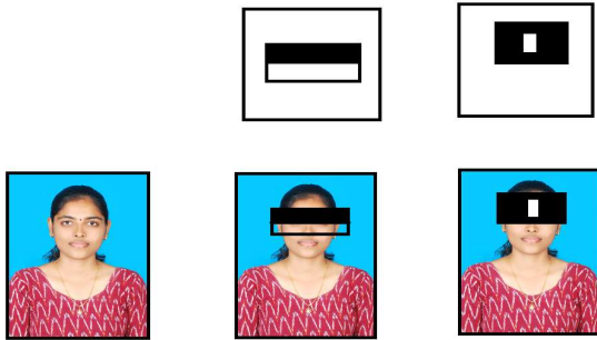
Figure 5.4 HAAR features applied to input image (Fig: 6.1)
