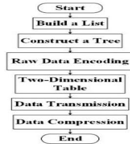
Figure 2: Flow Chart of Unbalanced Big Data Compression
