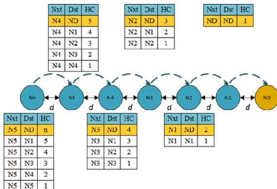
Figure 5 : Forward routing table in a conventional routing protocol.
