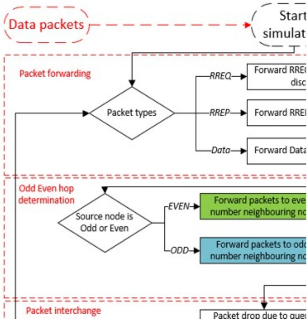
Figure 4 : AODVEO routing algorithm
