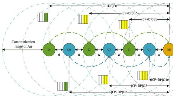
Figure 8: Packet accumulation flow in AODVEO.
