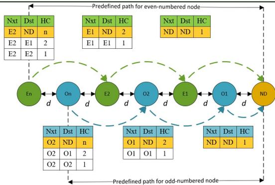
Figure 7: Forward routing table in AODVEO.
