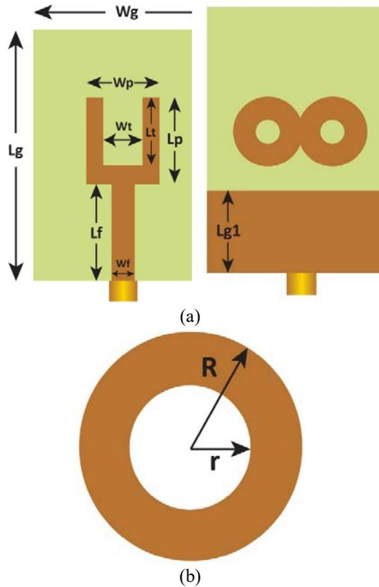
Fig 3. Antenna geometry of the proposed VBN-UWB [19]
