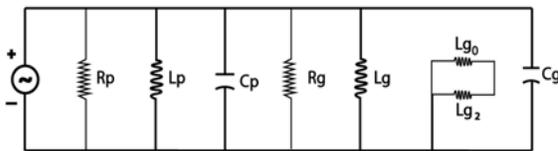
Fig 4. Rf Equivalent Circuit Of Vbn-Uwb
