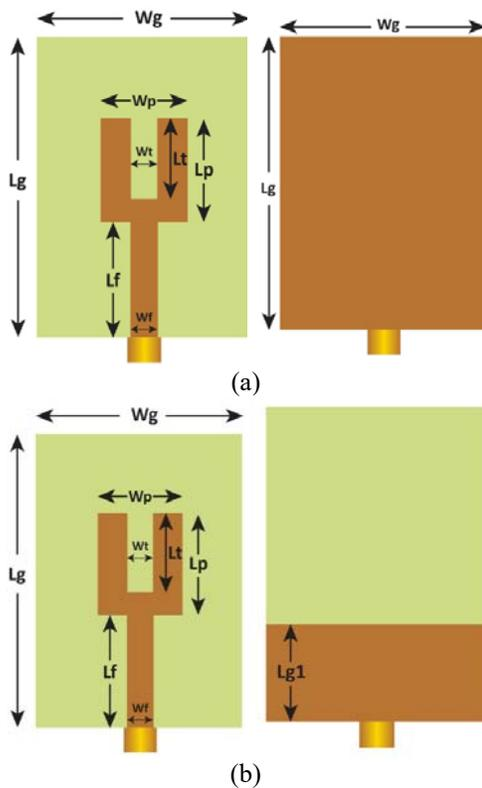
Fig 1. Antenna's Layout (A) TFS (B) PG-TFS [19]
