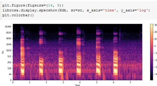
Figure 6: The Python code for converting an audio vowel signal for vowel /a/, /i/, /u/, /e/, /è/, and /o/ to a single spectrogram image, as well as an illustration of a spectrogram image at the bottom
