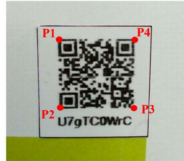
Figure 9: Visualization Example of Detected Four Quadrangle Points
