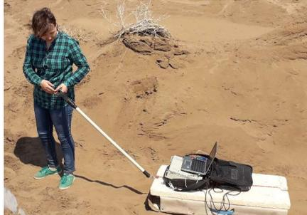
Figure 1: Zond-12e ground penetrating radar
