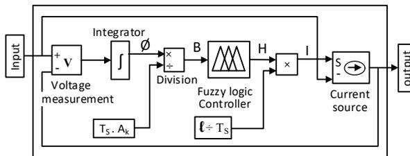
Figure 6: Equivalent Model Of A Non-Linear Inductance Under MATLAB-Simulink
