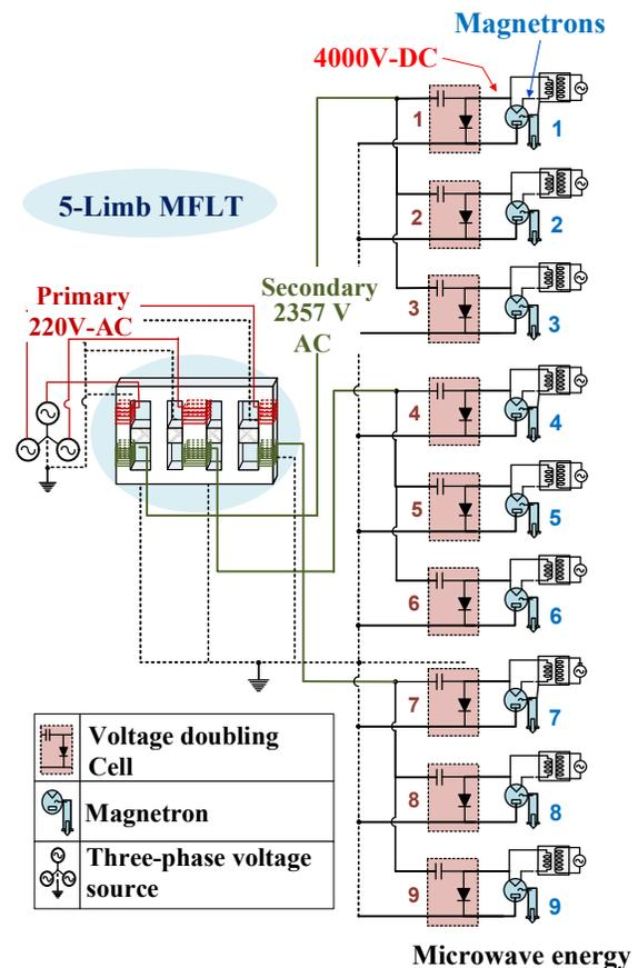
Figure 1: Design of the three-phase power supply of three MGTs per phase
