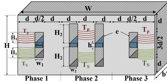
Figure 3: Design of the new 5-limb MFLT
