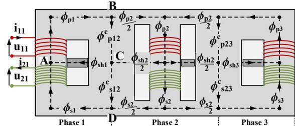
Figure 4: The flux distribution of the 5-limb MFLT
