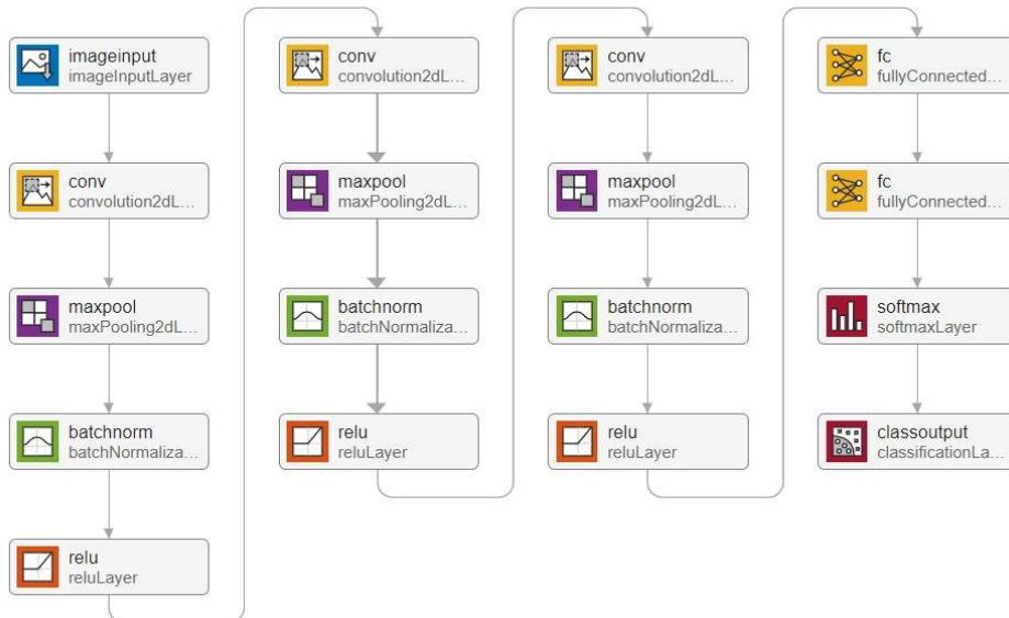
Figure 10: Description Of The CNN Layers Based Matlab
