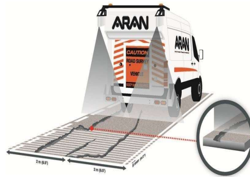
Figure 1. Laser Crack Measurement System Mounted On Mobile Car
