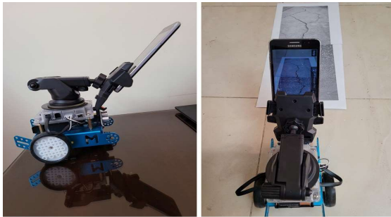
Figure 7 Proposed ARS system prototype for pavement crack detection
